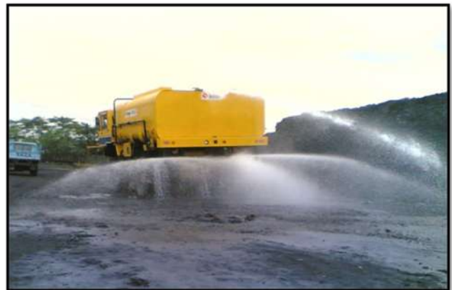
Mobile sprinkling for dust suppression at Ananta OCP
